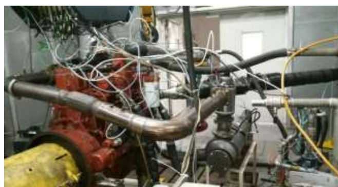
Figure 2-5 Test bench for diesel engine of China phase V.
